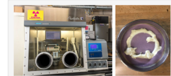
Radon Diffusion Test Chamber and a test sample
